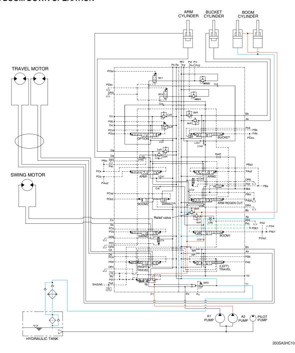
When the right control lever is pushed forward, the boom 1 spool in the main control valve is moved to the down position by the pilot oil pressure (PBb1) from the remote control valve.
