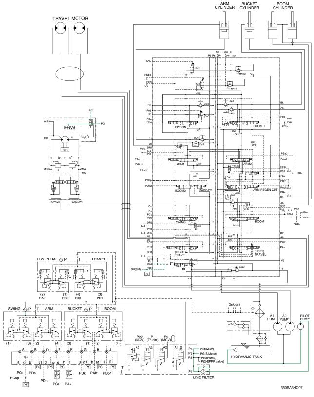
When one of the RCV lever (except travel lever) is tilted, the pilot oil flows into SH port through main control valve.
